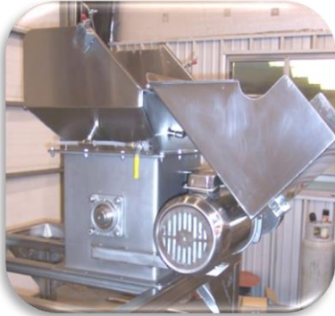
Chopper Shown with Safety Hood in Open Position
