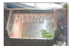
Filters Particles out 1/32" and Larger
